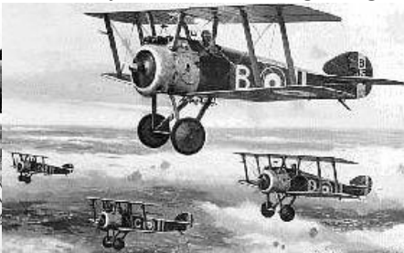
Sopwith Camel RFC / RNAS / RAF with its twin .303" Vickers MMG's
