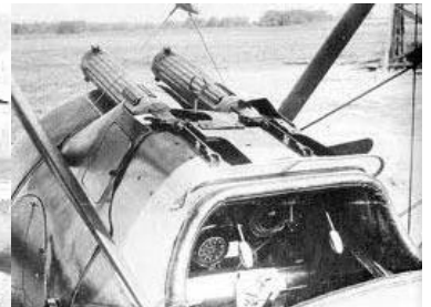
Sopwith Camel RFC / RNAS / RAF with its twin .303" Vickers MMG's
